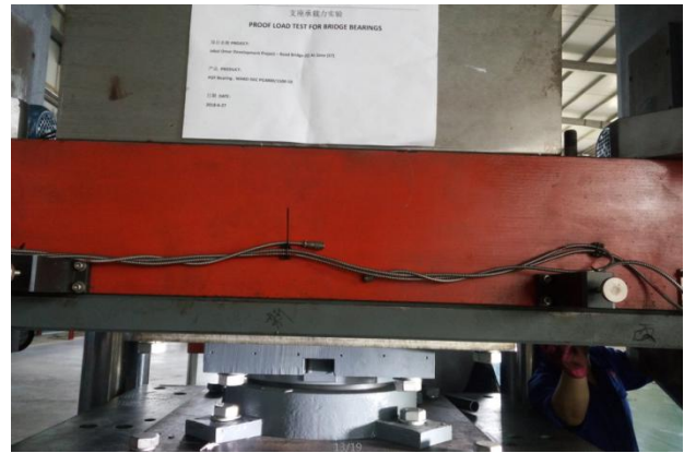
Proof load test of pot bearings as routine test prior to shipment
