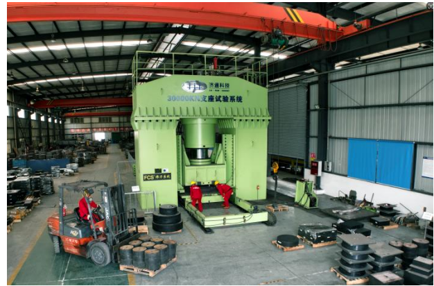
IEC's shear-compression tester with 30000kN vertical load
