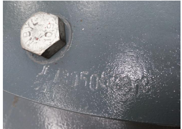
Stenciled traceability NO. on POT
