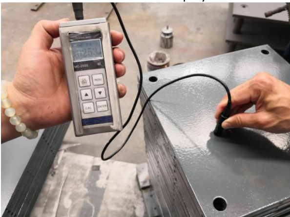
Measurement of thickness of the dry film of paint
