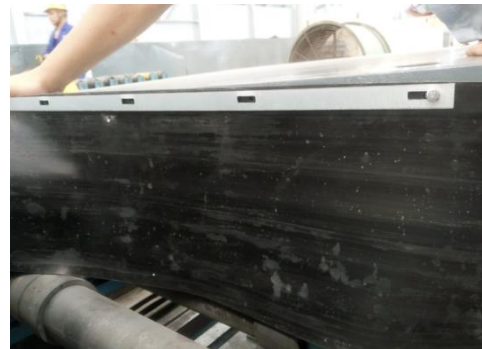
assemble the dustproof cover by screw
