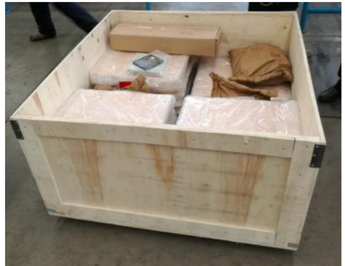
pot bearings packed in wooden frame catered for sea-shipping
