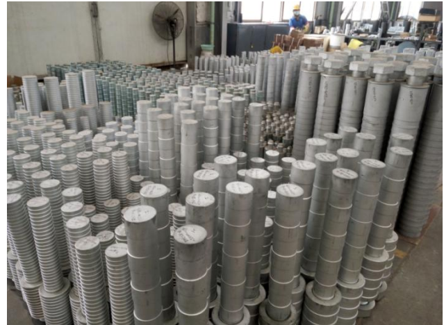
Dacromet treated bolts/sockets
