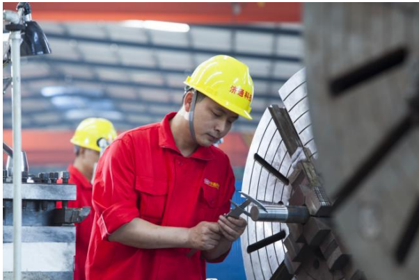
Workshop workers carefully checking the dimension of bearing parts during fabrication process
