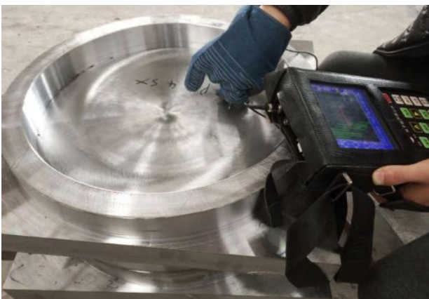
UT NDT testing on the POT of Pot Bearing
