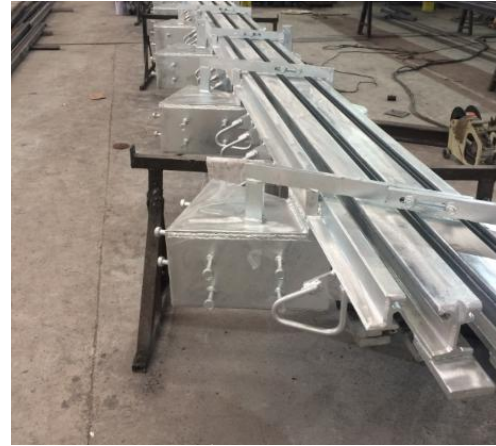
Hot-dip-galvanized treatment for NOH2 project in Doha Qatar, 2018
