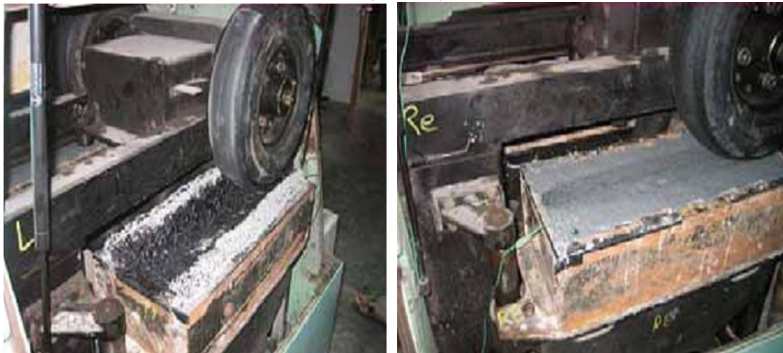
Test pieces of PUF-80 with a length of 1m were tested in-house with contact pressure of 0.95\text{MPa} , 150\text{kN} loading. Max. Doformation was measured less than 0.5\text{mm} .
