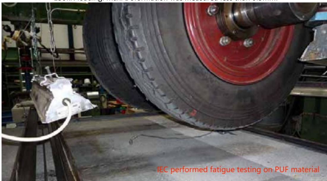
IEC carried out type testing of full PUF joint assembly subject to scenario simulating
