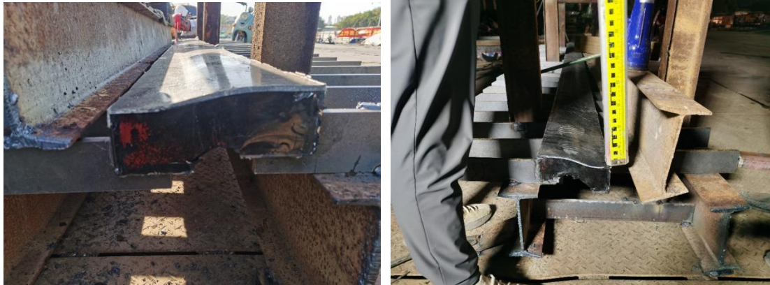
Test pieces of PUF-80 and PUF-100 with a length of 4m were tested at shear movement of \pm 40\text{mm} under open temperature 35^\circ\text{C}
