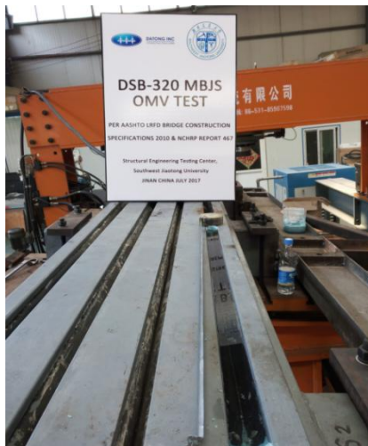
OMV and SPO test setup for IEC's modular expansion joint according to AASHTO LRFD Bridge Construction Specifications and NCHRP Report 467
