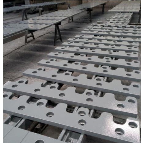
Painting of finger expansion joint at IEC for Tama Bridge over Nile, Egypt, 2019
