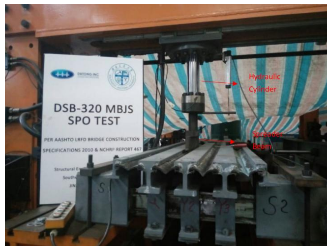
OMV and SPO test setup for IEC's modular expansion joint according to AASHTO LRFD Bridge Construction Specifications and NCHRP Report 467
