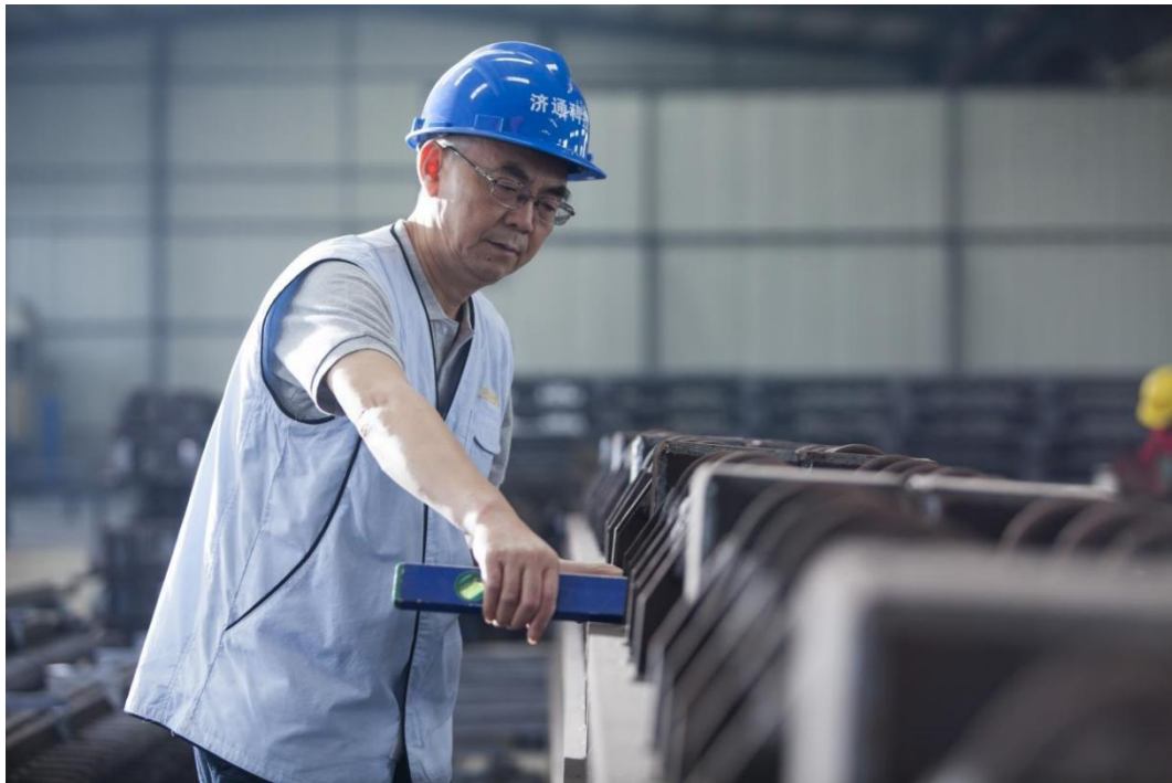
IEC QC controller is working on a modular joint for dimension checking
