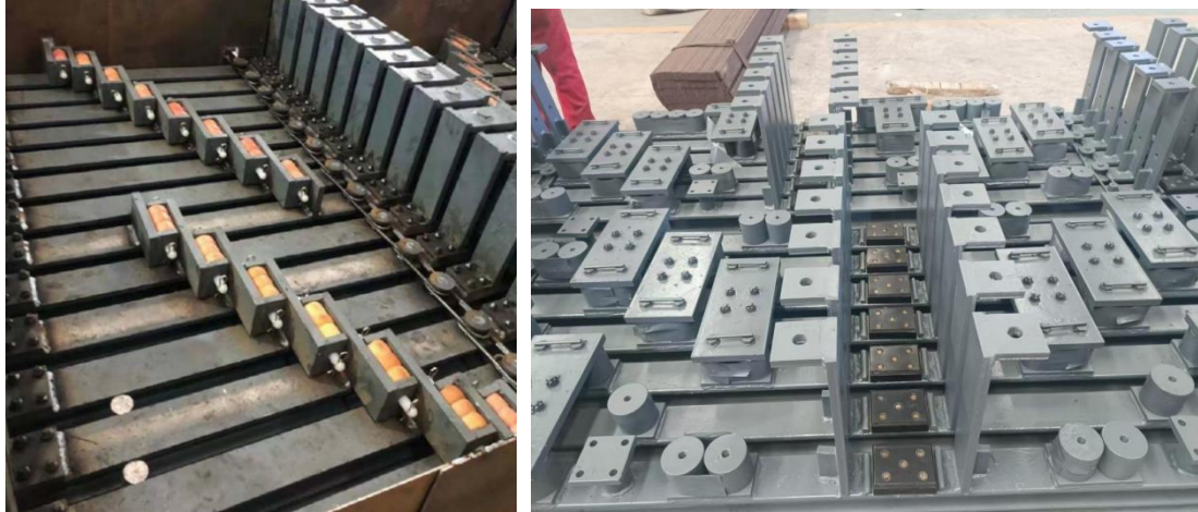
Different layouts of control springs alignment in differently-sized modular expansion joint (right: control springs behaviour after Opening Movement with Vibration test Left: control springs layout in a 14-cell MBJS for Hulukou Bridge over Jinsha River, Yunnan, China)
