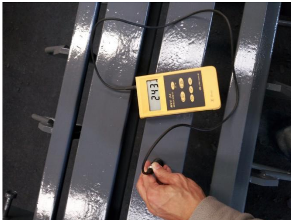
paint film thickness 243 microns (C5-MI) for E-ring road project in Doha Qatar, 2018
