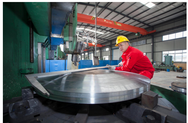
IEC's staff is measuring dimension of convex plate of a spherical bearing
