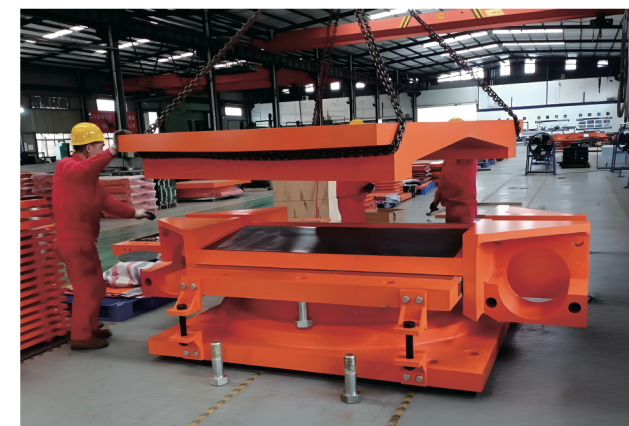
Specially-designed Self-aligning Slope Bearing was assembled for Mazhu Expressway, Hubei Province, China
