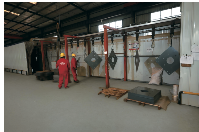
IEC's Auto-rotating spray line for paint as corrosion-resistance
